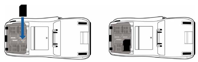
Figure 16 Inserting SIM Card
